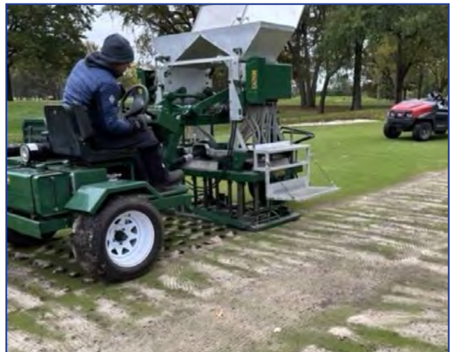
Drill & Fill Process
